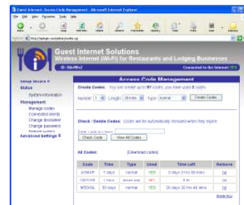
Access codes are generated and managed using a simple display
